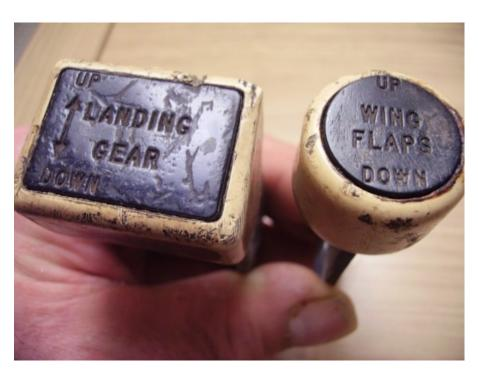
The images show one of the first human factorsdriven changes to airplane controls. Pilots would frequently activate the wrong controls upon landing. To avoid this, critical controls were given different shapes and feels. These controls are for a plane designed in 1939 and used in WWII starting in 1942.
